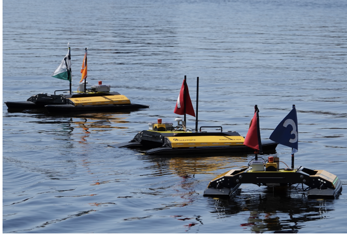
Fig. 4: The Clearpath Robotics Heron USVs are used for testing these controllers on the water.
